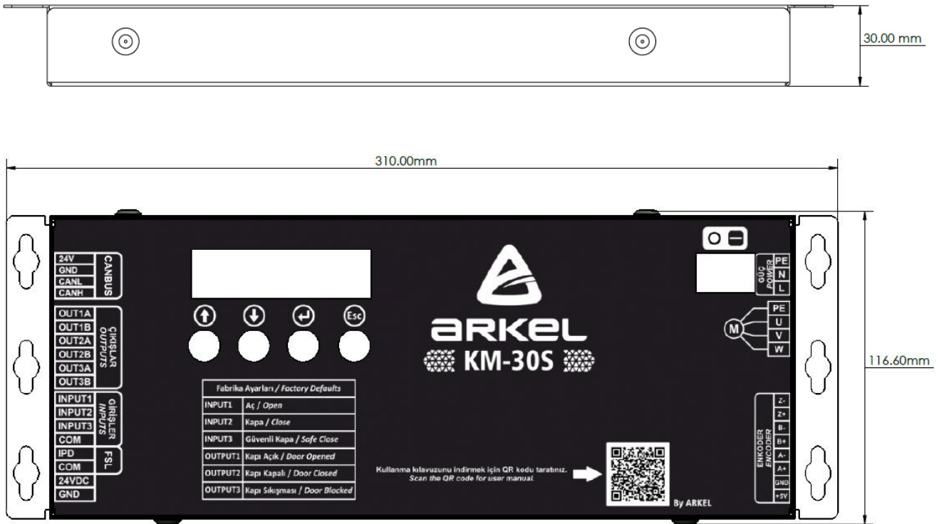
Figure 13 Length x Width x Height of KM-30S
